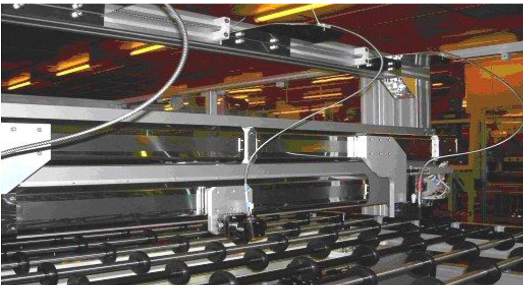
In-line chromaticity and thickness measurement in display production
