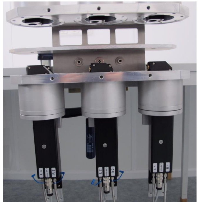
Full 3-channel reflectance-setup for inline thickness control
